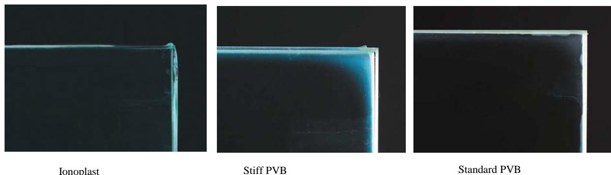
Fig. 4 Laminates after 3000 Hours of Salt Spray
