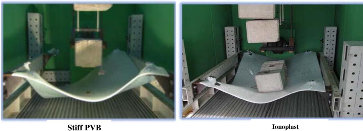
Fig. 3 Stiff PVB 1.52 mm and Ionoplast 0.89 mm
